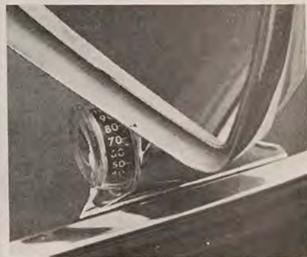
The Cadillac's rotating dial outside thermometer.
