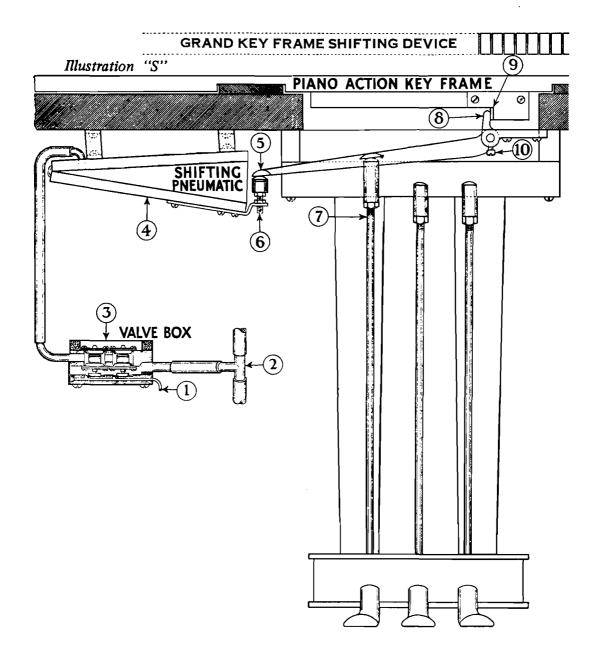
Above illustration, "S," shows the grand key frame shifting device; this was installed only in the late model grand Duo-Art.
