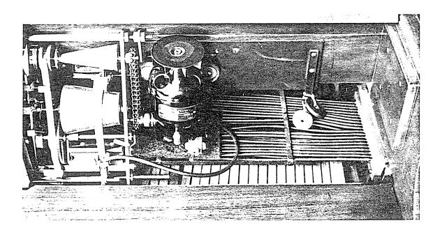
Right side of spool box, 1932 Steinway Duo-Art. Electric roll drive, with reversible cone drive tempo device.
