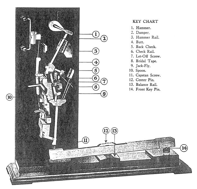
No. 10. Block off the loud pedal to distance that spoon lifts dampers. Block off soft rail about 1 inch from strings. Regulate bridal tapes No. 8 so that all slack is taken out of tape when soft rail is up to 1 inch from strings.
