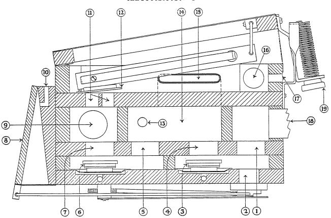
With the "Dynamic Lever" in front of Duo-Art at the "Concert" or normal position, the modulator valve No. 6 is open and allows the air entering chamber No. 9 to pass down through channel No. 7, then up through channel No. 5 into chamber No. 14, where it passes down channel No. 4 and up channel No. 1 to outlet No. 18, then it passes to the pump and is exhausted.
