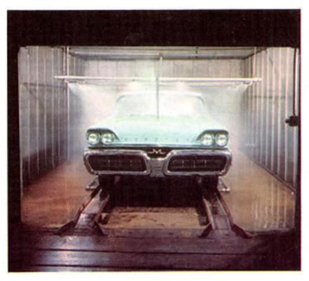
TO MAKE SURE IT'S WEATHERTIGHT, a '58 Mercury undergoes a high-velocity shower bath as part of the Mercury Quality Audit program.
