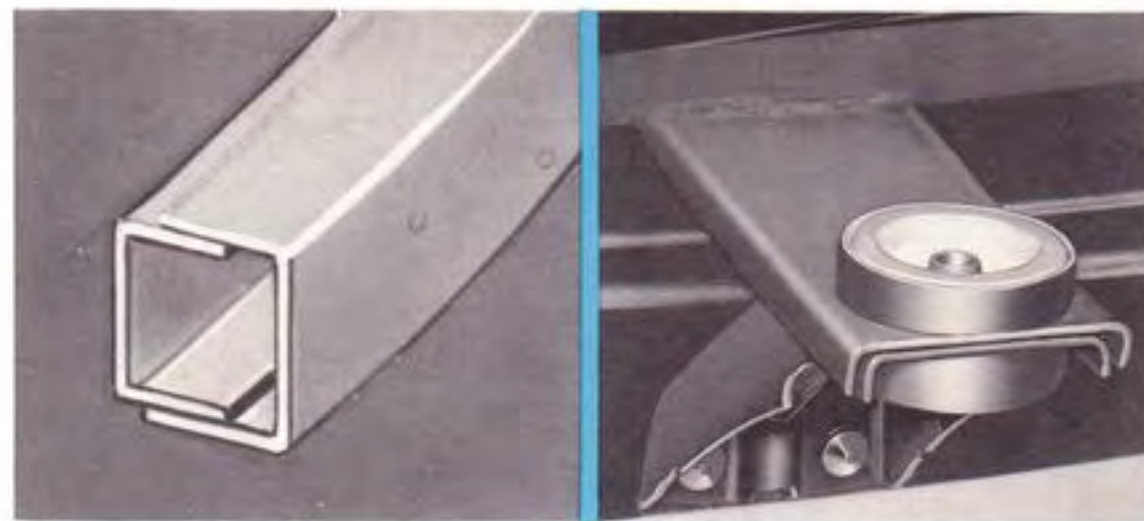
Frame features illustrated above are: Mercury's basic frame showing ladder-type construction and outward curved side rails, the X-type reinforcement for convertible frames, and the special tubular cross-member for station wagon frames. In the lower illustrations are a cross-section of the welded side rails showing wide overlap of the inner and outer U-channel members, and a rubber body mount installation.
