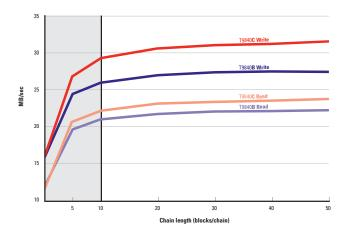
Figure 6 was created using an EXCP application in which the chaining length was explicitly specified. However, coding DCB=BUFNO=nnn in DD statements can be used with several of the other access methods to control the chain length of channel programs. This is accomplished indirectly by specifying the number of buffers used by the access method. For example, QSAM will, on average, transfer BUFNO/2 blocks per I/O operation from the application.
