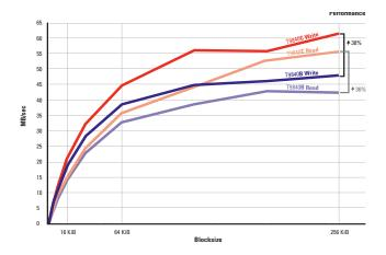
Figure 4 can also be used to estimate the performance of applications based on their blocksizes. Table 1 lists some applications and their respective blocksizes. Note that maximum performance can be achieved using large block applications such as StorageTek's Extended High-Performance Data Mover (ExHPDM) software.
