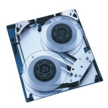
The T9840C provides backwards-read compatibility in that it can read cartridges written on T9840A and T9840B tape drives to facilitate migration to the T9840C recording format. Cartridges rewritten on the T9840C are automatically written at the higher recording density.
