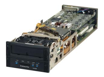
Like the T9840C tape drive, the T9940B has a similar 30 megabyte-persecond native head-to-tape speed and similar FICON interface. As a result, the T9940B FICON drive throughput is nearly identical to the T9840C FICON drive (Figure 14).
