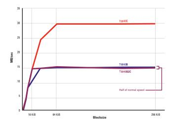
Figure 12 shows the same combination of scenarios at various levels of data compression. It can be seen that with 4:1 compression or better, the T9840C is able to achieve native read performance while reading in compatibility mode at the lower density.
