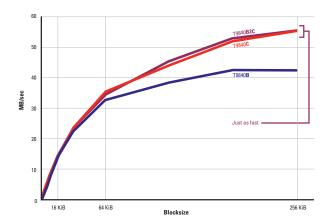
Figure 11 shows the same scenarios using uncompressable or 1:1 data compression. Here we see that the T9840C reads the T9840B cartridge at about one half of normal speed. This fits with expectations, because the data on the T9840B is written at about one half the recording density as a native T9840C.
