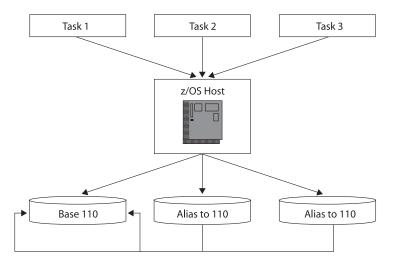
PAV assigns "aliases" to the base device, in effect creating multiple concurrent I/O ports for data requests.
