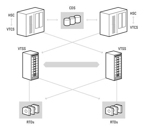
Clustered VTSS adds the further replication of VTVs to a secondary VTSS, which reduces the time required to restore the contents of a failed VTSS buffer.
