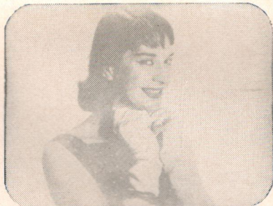
Picture too light —inadequate contrast. Increase Contrast control setting. Decrease Brightness control setting if necessary.
