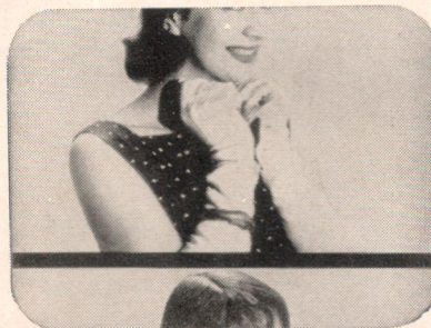
Picture moving up and down —Vertical Hold control incorrectly adjusted.
