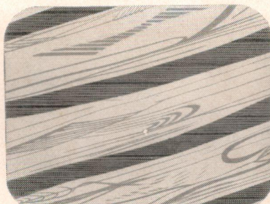
Diagonal lines or stripes across picture —Horizontal Hold control incorrectly adjusted. Turn the Horizontal Hold control clockwise until a steady picture is obtained.
