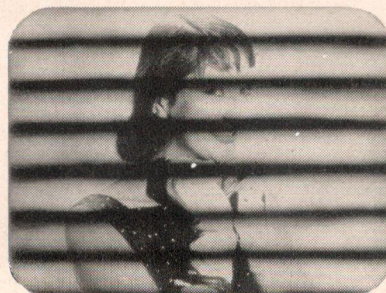
Sound bars on picture —Adjust Fine Tuning control.
