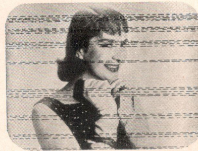
Electrical Interference —as from electric drill or household appliance.
