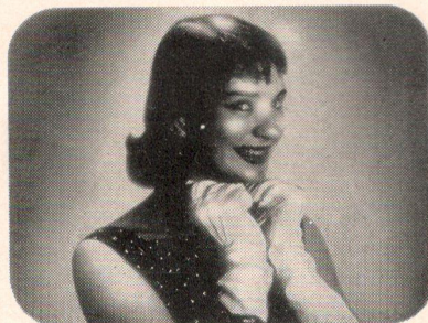
Picture too dark —excessive contrast. Reduce Contrast control setting. Increase Brightness control setting if necessary.
