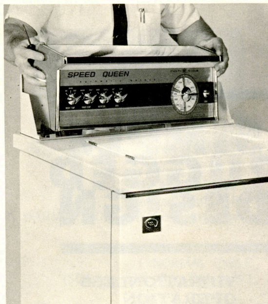
Removal of 2 screws permits control panel to be detached so that back side of panel is exposed for servicing.
