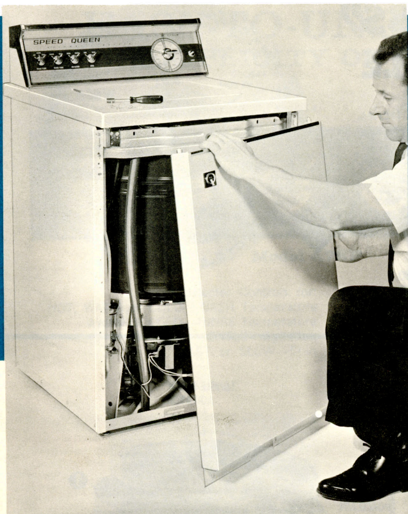
Removal of 4 screws across bottom is all that is necessary to take off front panel.
